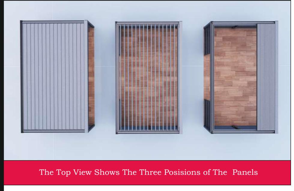
The Top View Shows The Three Positions of The Panels
