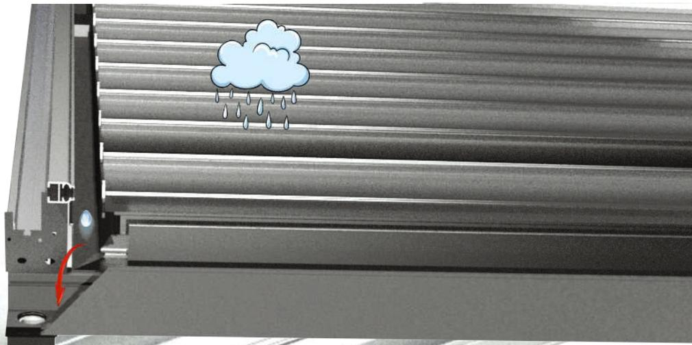
The Path of Rainwater and Snow From the Panel to the Outside
